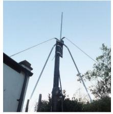
The four quarter wave ground planes are bent downward to produce a feed impedance of about  $50\Omega$  to match the coax.
