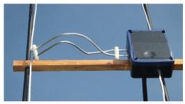
The three directors were made from aluminium rod (I used 3mm welding rod bought in a pack of 50 from EBay). I have a long length of 4mm diameter aluminium wire in my cupboard for years doing nothing so I used it to make the
